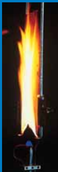
Vertical flame test on non-flame resistant fabric.
